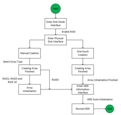
Figure 13-1 RAID Working Flow
