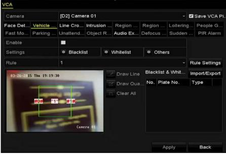
Figure 10-3 Set Vehicle Detection
