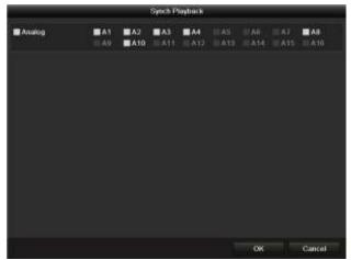
Figure 6-7 Select Channels for Synchronous Playback
