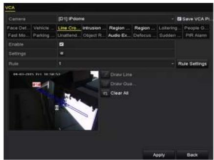
Figure 10-6 Draw Line for Line Crossing Detection
