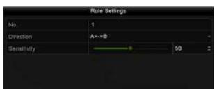
Figure 10-5 Set Line Crossing Detection Rules
