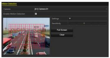
Figure 5-15 Motion Detection- Mask
