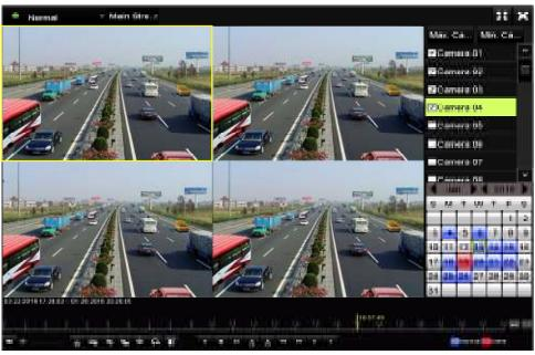
Figure 6-25 4-ch Synchronous Playback Interface
