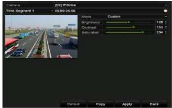
Figure 15-6 Image Settings Interface (IP Camera)
