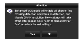
Figure 17-10 Enable Enhanced VCA Mode
