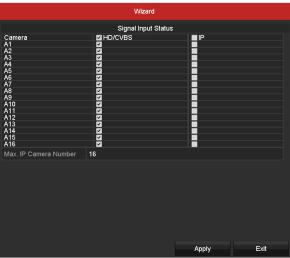
Figure 2-15 Configure Signal Input Type
