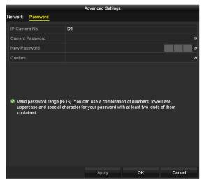
Figure 2-45 Password Configuration of the Camera
