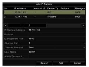
Figure 2-28 Quick Adding IP Camera Interface
