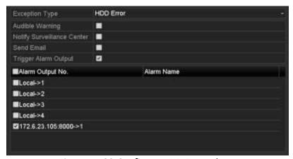
Figure 14-29 Configure HDD Error Alarm
