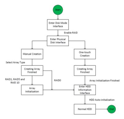
Figure 13-1 RAID Working Flow
