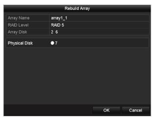
Figure 13-12 Rebuild Array Interface
