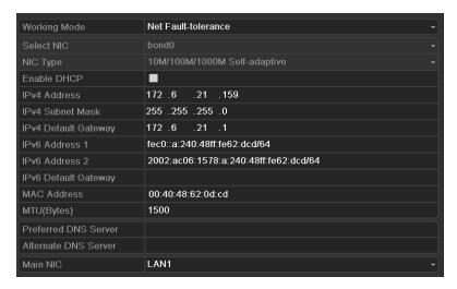
Table 12-1 Net Fault-tolerance Working Mode
