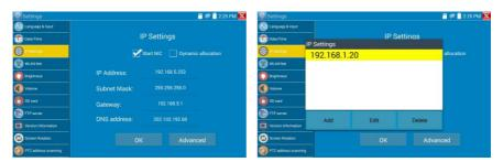
After setting an advanced IP address (refer to the photos above), the unit can test two network segments (192.168.5.0) and (192.168.1.0).
