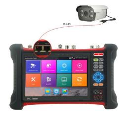
Note:1) If the IP camera requires PoE power, then connect the IP camera to the IP tester's LAN port.
