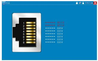
Connect a network cable from a PoE switch to the IP tester's PSE IN port. Connect an IP camera or other PoE using node to IP tester's LAN port, the PoE voltage and the cable's pin connection status show on the screen.
