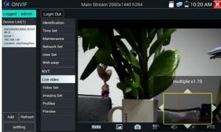
When the image is enlarged, if not operate on touch screen, it can operate by the keyboard press the key to zoom in , press the key to zoom out press upward and downward key to move image.
