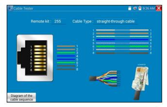
Test LAN cable or telephone cable.
