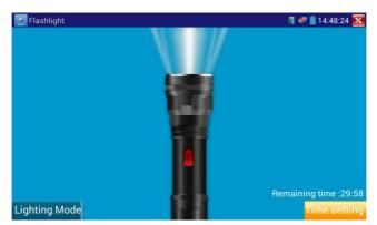
While in the flashlight app, click the red button to turn on the LED lamp. Press it again to turn it off. If you don't press the red button to shut off the lamp and press the button to exit the app, the lamp will stay on. Click the Time Setting button to set a timer that will shut off the lamp.
