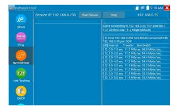
Network bandwidth testing can also be tested with a computer using compatible network bandwidth testing software. Install network bandwidth testing software on a computer, as a test Client or Server, to do the mutual testing with the tester. If use computer as the server, the computer IP address is :192.168.0.39
