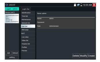
**Network setting:** Click "Network Set "to change the IP address. Some cameras cannot support change IP address, so there is no change after saving.
