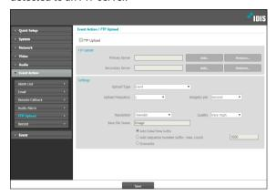
• FTP Server: Click Add to register a new FTP server. Click Remove to remove a registered FTP server. When an event is detected, a .jpg image of the event detected image is uploaded to the Primary Server. If the upload to the Primary Server fails, the file will be uploaded to the Secondary Server. Upload to the Secondary Server will continue to be attempted until successful. Fill out the fields below and click Test to test the FTP server connection settings. Once the test is complete, click OK.
