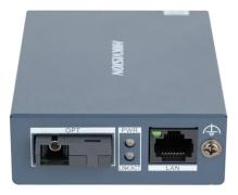
DS-3D501R-A is a gigabit single-mode single-fiber fiber optical transceiver developed by Hikvision. It provides one 10/100/1000 Mbps self-adaptive RJ45 port and one 1000 Mbps SC fiber optical port, and can achieve high-speed and lossless transmission of data signals over a maximum of 20 km transmission distance.
