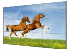
The DS-D2046TL-1B LCD display uses an industry-level ultra-narrow bezel design, which enables a bezel width of 2.5 mm between neighboring displays. The adopted direct-lit LED backlighting technology helps achieve ultra-high and uniform brightness of 500 cd/m<sup>2</sup> without boundary shadows. The display has abundant interfaces for video inputs, such as DVI, VGA, HDMI, and DP.
