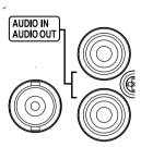
Connect the audio device to the **AUDIO IN** port and speakers with a built-in amplifier to the **AUDIO OUT** port. Use the **AUDIO OUT** port to listen to audio from analog cameras.
