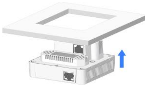
Figure 1-12 Push AP into Groove
