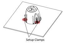
3 Fix the top cap magnetically onto the speaker body.
