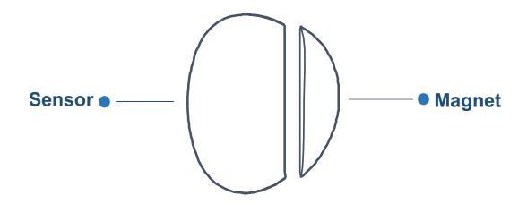
This sensor is magnet based. When the main body and the magnet are separated beyond a certain distance (about 1 inch), it notifies the BOSMA X1 camera it is paired with.
